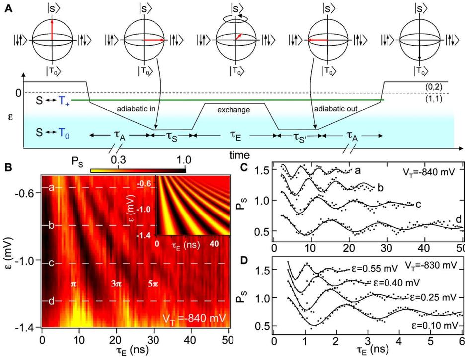
FIG. 48. (Color online) Coherent two-electron spin state rotations. (a) Pulse sequence. (b) Singlet state probability  $P_S$  measured as a function of the pulse time  $\tau_E$  and detuning  $\epsilon$ . (c) Horizontal cuts through the data in (b) show clear oscillations in  $P_S$ . (d) By increasing the tunnel coupling, a fast  $\sqrt{\text{SWAP}}$  operation time of  $\sim 180$  ps is achieved. Data reproduced from [Petta, Johnson, Taylor, \*et al.\*, 2005](#).
