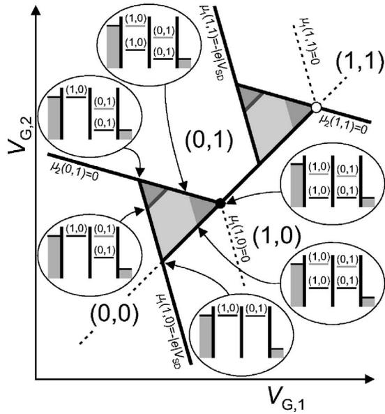
FIG. 30. The triple points for an applied source-drain bias  $V_{SD}$  and the drain kept at ground. A triangle is formed from each triple point. Within this bias triangle charge transport through the dot is energetically allowed. Gray lines and regions in the triangles illustrate the gate voltages at which transitions involving excited-state levels play a role. Electrochemical potentials corresponding to transitions involving an excited state are shown in gray in the level diagrams.
