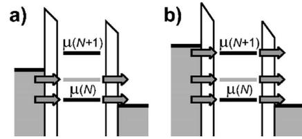
FIG. 4. Schematic diagrams of the electrochemical potential levels of a quantum dot in the high-bias regime. The level in gray corresponds to a transition involving an excited state. (a) Here  $V_{SD}$  exceeds  $\Delta E$  and electrons can now tunnel via two levels. (b)  $V_{SD}$  exceeds the addition energy for  $N$  electrons, leading to double-electron tunneling.
