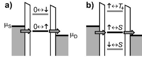
FIG. 10. Few-electron quantum dot operated as a bipolar spin filter. Schematic diagrams show the level arrangement for ground-state transport at (a) the  $0 \leftrightarrow 1$  electron transition, where the dot filters for spin-up electrons, and (b) at the  $1 \leftrightarrow 2$  electron transition, where the dot only transmits spin-down electrons.
