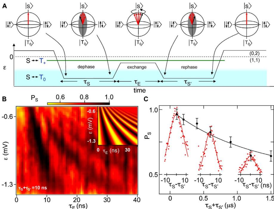
FIG. 49. (Color online) Error correction. (a) Singlet-triplet spin-echo pulse sequence. (b) Singlet state probability  $P_S$  measured as a function of pulse time  $\tau_E$  and detuning  $\epsilon$ . Clear singlet state recoveries are observed for  $\pi$ ,  $3\pi$ ,  $5\pi$  exchange pulses. (c) The singlet state recovery persists out to  $T_2 = 1.2 \mu\text{s}$ . Data reproduced from [Petta, Johnson, Taylor, \*et al.\*, 2005](#).
