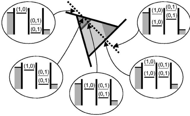
FIG. 31. Level diagrams for different detunings  $\epsilon$  between dot 1 and dot 2 (dotted line in the bias triangle). Note that the average of the levels in the two dots is kept constant, and only the difference between the levels is changed.
