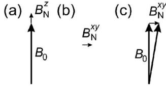
FIG. 25. Longitudinal magnetic-field fluctuations  $B_N^z$  add directly to the external field  $B_0$ , whereas transverse fluctuations  $B_N^{xy}$  change the total field only in second order when  $B_0 \gg B_N^{xy}$ .
