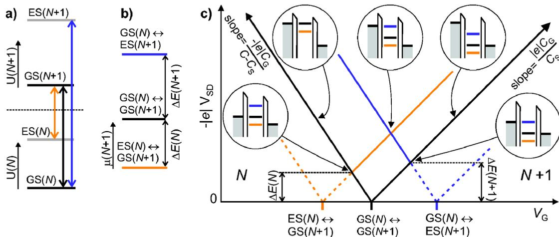
FIG. 5. (Color online) Schematic of a high-bias measurement. (a) Energies for  $N$  electrons  $U(N)$  and for  $N+1$  electrons  $U(N+1)$ . Possible transitions are indicated by arrows. (b) The electrochemical potential ladder for the transitions depicted in (a). (c) Schematic plot of the differential conductance  $dI_{\text{DOT}}/dV_{SD}$  as a function of  $-|e|V_{SD}$  and  $V_G$ . At several positions the level alignment is indicated with schematic diagrams.
