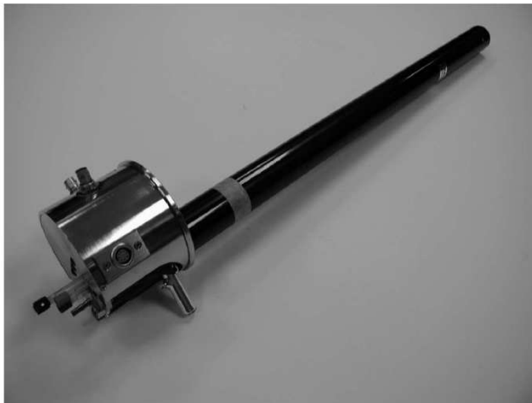
Figure 3-4: The above probe is a Nalorac HFX probe, where X was tuned to ^{13}\text{C}
