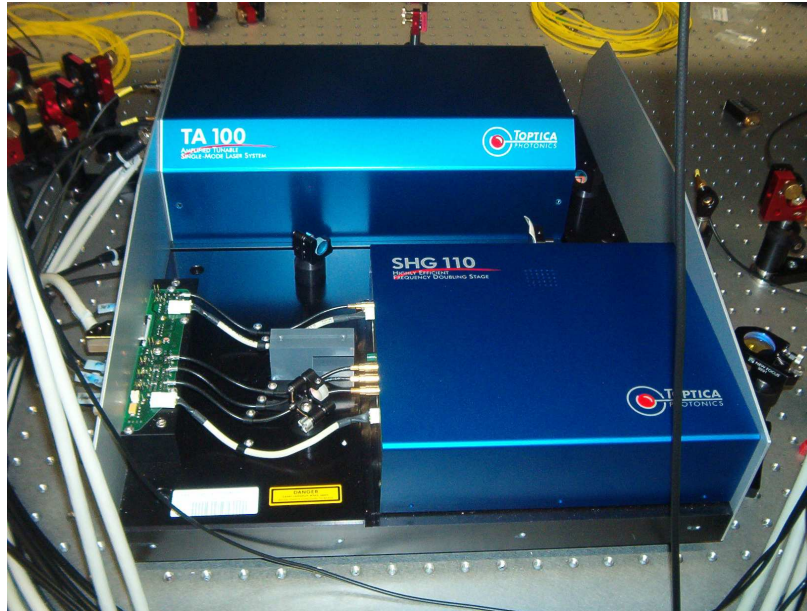
Figure 9-3: Photograph of the 397 nm laser. The main laser diode is contained within the larger box, while the doubling cavity is within the smaller. The distance between holes on the optical table is 2.5 cm.
