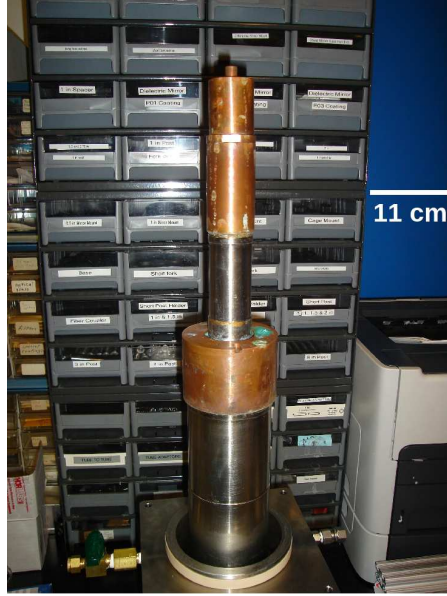
Figure 7-16: Photograph of the expander. This unit had been removed due to a helium leak. Some corrosion is visible, which may be due to the presence of liquid water if the bellows had not been adequately flushed with helium.
