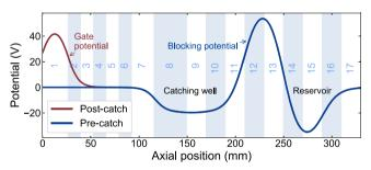
Fig. 6 Potentials on-axis for Be $^+$  capture and stacking. Shaded and numbered regions represent electrode positions. Ions enter from the left into the blue potential. Subsequently, the gate electrode (E1) is raised to  $40\,\mathrm{V}$  (red potential) to capture them. Ions are then moved to the reservoir where they are combined with previous loads and laser-cooled until the desired number of stacks have been accumulated.
