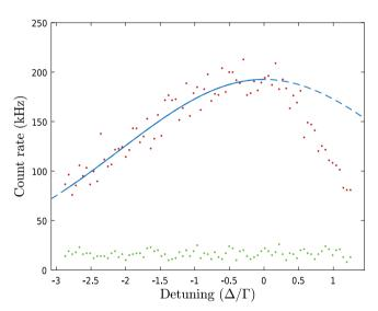
Fig. 10 Fluorescence signal from a pure  $Be^+$  plasma as the frequency of the cooling laser is scanned across the laser cooling transition. The
