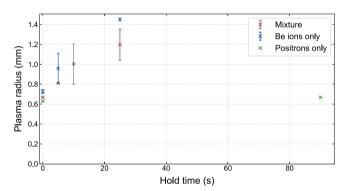
Fig. 8 Evolution of the radius of three different plasmas as a function of time without laser-cooling in a 1 T field. The mixture (red) consists of  $2.6\times10^6$  e $^+$  and  $4\times10^5$  Be $^+$ . The Be $^+$  only plasmas contained  $4\times10^5$  Be $^+$ . The positrons only plasma contained  $2.6\times10^6$  e $^+$ . The vertical error bars correspond to the standard error on the mean radius measured at each hold time.
