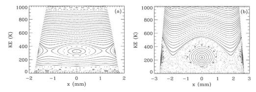
**Figure 5.** Same as figure 4 except using the much simplified map which consists of rotations and small translations. Note the very similar structure for the corresponding case in figure 4. For this map, the kinetic energy is defined as  $KE(r) = KE(0) - en_0 r^2/(4\epsilon_0)$ .
