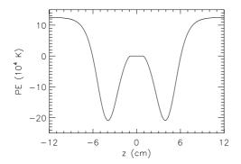
**Figure 1.** The electric potential energy for a  $\bar{p}$  along the trap axis. The flat region near 0 cm is where the e<sup>+</sup>'s are trapped with 0 being the centre of the e<sup>+</sup> plasma. This simulation has the e<sup>+</sup>'s at 4 K with a density of  $n_0 = 1.2 \times 10^7$  cm<sup>-3</sup> and for  $8 \times 10^6$  e<sup>+</sup>'s. The plasma is roughly a spheroid in shape with a radius of 4.33 mm and a length along the axis of 17.1 mm. The mirror coils are at  $\pm 12$  cm.
