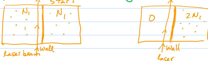
excited atoms get through wall; ground state atoms bounce off wall; laser excites atoms just before wall
