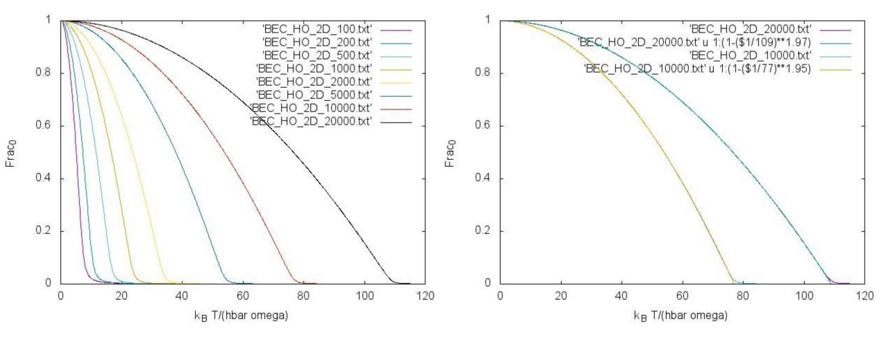
The left plot is fraction of atoms in ground state, right plot is a "by eye" fit to the fraction There is a clear transition that becomes sharper with increasing N Fraction is proportional to  $1 - (T/T_C)^2$  with  $T_C$  proportional to the square root of N
