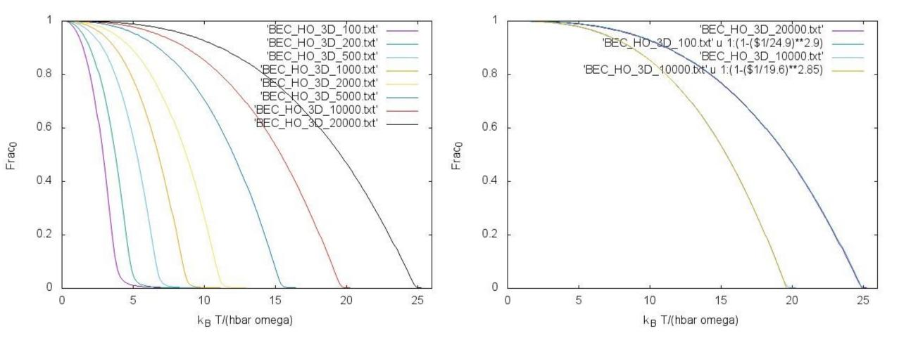
The left plot is fraction of atoms in ground state, right plot is a "by eye" fit to the fraction There is a clear transition that becomes sharper with increasing N Fraction is proportional to  $1 - (T/T_C)^3$  with  $T_C$  proportional to the cube root of N
