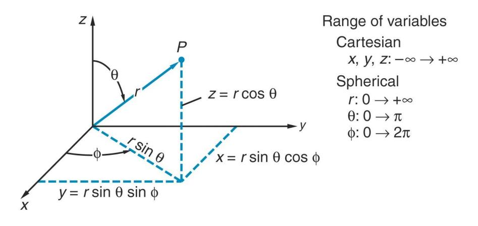
$$\frac{\partial^2 F}{\partial x^2} + \frac{\partial^2 F}{\partial y^2} + \frac{\partial^2 F}{\partial z^2} = \frac{1}{r^2} \frac{\partial}{\partial r} \left( r^2 \frac{\partial F}{\partial r} \right) + \frac{1}{r^2 \sin(\theta)} \frac{\partial}{\partial \theta} \left( \sin(\theta) \frac{\partial F}{\partial \theta} \right) + \frac{1}{r^2 \sin^2(\theta)} \frac{\partial^2 F}{\partial \phi^2}$$
