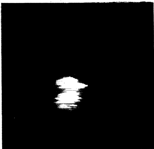
FIG. 7. Image ( 303\times 303 Å) inside the flat region in Fig. 6. The bright hill is around 80 Å in diameter and 8 Å in height. The underlying ordered structure is the same as in Fig. 4, with a z corrugation of about 0.8 Å.
