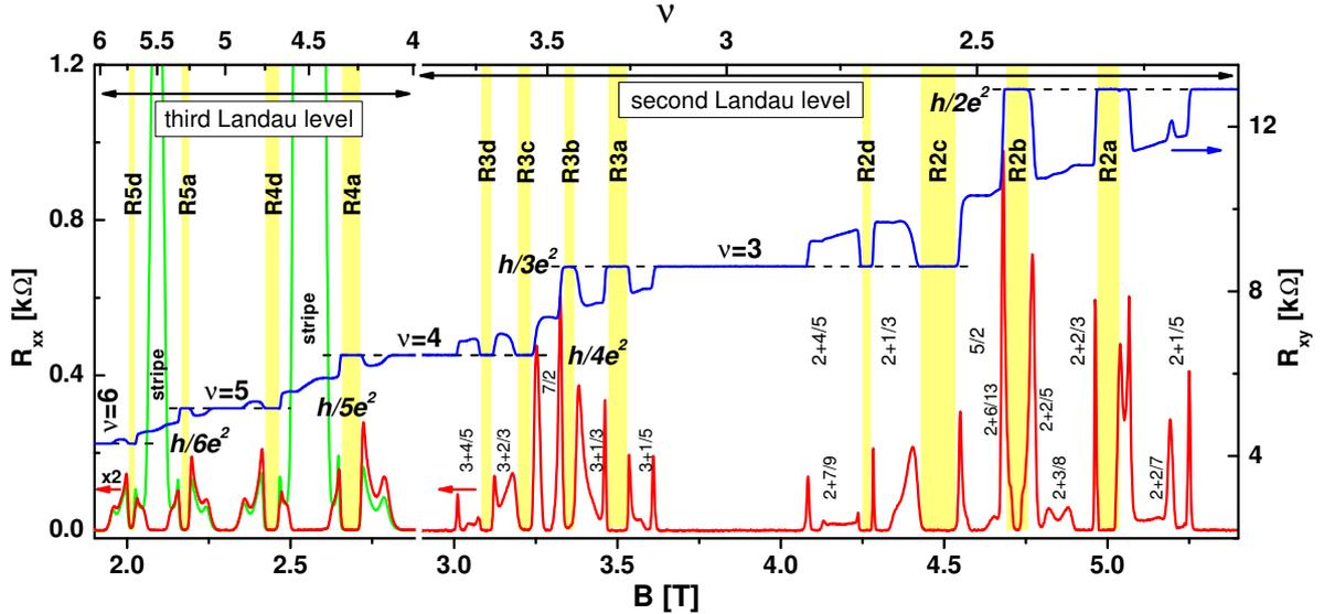
FIG. 1. The magnetoresistance in the second ( $2 < \nu < 4$ ) and third ( $4 < \nu < 6$ ) Landau levels as measured at 6.9 mK and 77mK, respectively. RIQHSs are marked by shaded stripes and FQHSs by their filling factors. In the TLL the two  $R_{xx}$  traces shown are measured along mutually perpendicular directions and, for clarity, are magnified by a factor two.
