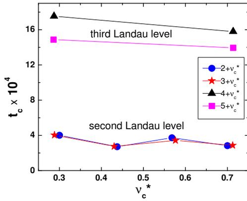
FIG. 4. The reduced onset temperatures  $t_c = k_B T_c / E_c$  of the RIQHSs in the SLL and TLL plotted as function of the partial filling factor  $\nu_c^*$ . Lines are guides to the eye.
