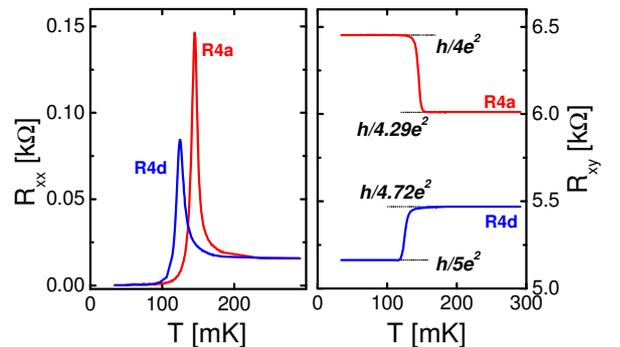
FIG. 3. The magnetoresistance  $R_{xx}$  and the Hall resistance  $R_{xy}$  of two RIQHSs in the third Landau level measured at  $\nu = 4.29$  and  $\nu = 4.72$ .
