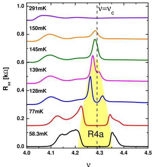
FIG. 2. The evolution with temperature of the  $R4a$  RIQHS of the third Landau level. For clarity traces are shifted by  $150\Omega$  relative to another and the reentrant region is shaded.
