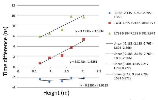
Speed measured using counters 1 and 3:  $v_{13}=\left(\frac{1}{3.315}\right)m/ns=3.0\times10^8~m/s$ Speed measured using counters 1 and 4:  $v_{14}=\left(\frac{1}{3.154}\right)m/ns=3.2\times10^8~m/s$
