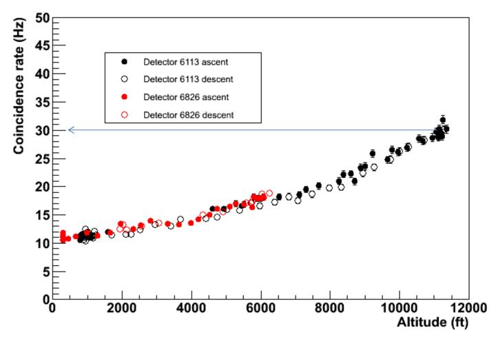
The rate changes by a factor of 3 over a distance of about 11000 feet (3350 meters)
