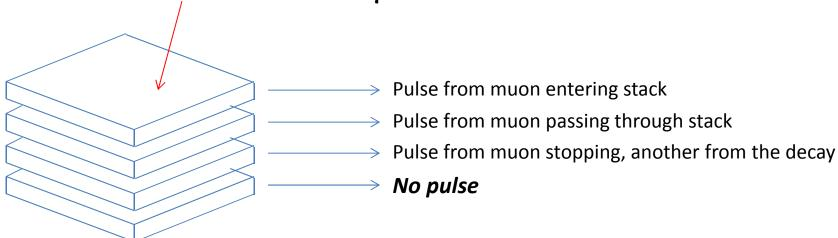
Require 3-fold coincidence GATE WIDTH = 10,000 ns PIPELINE DELAY = 20 ns This isn't *exactly* what we want because it triggers on any 3 channels, but the trigger rate is low enough that we can examine each event to see if it is just the top three channels with pulses.
