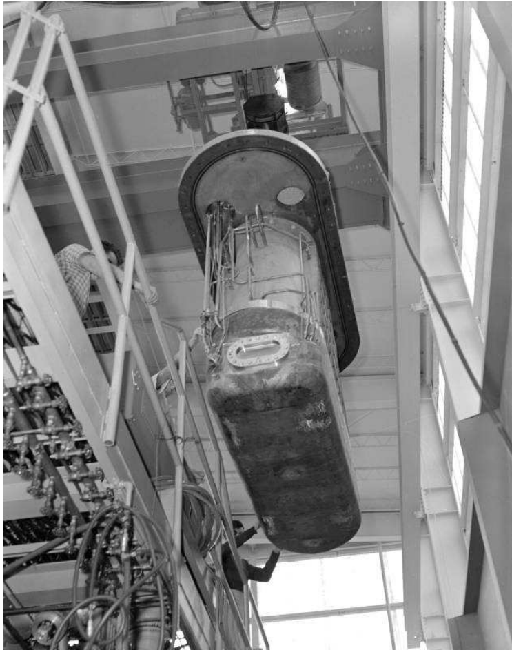
The Berkeley 72 inch liquid hydrogen bubble chamber
