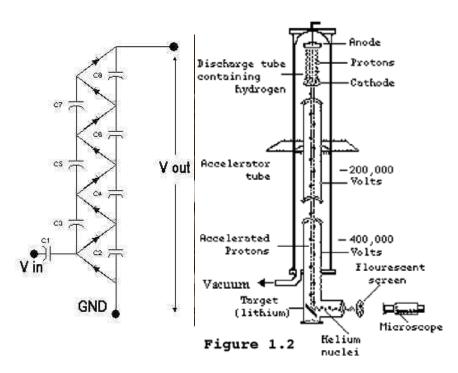
In 1932, Cockroft and Walton accelerated protons to 600 keV, produced the reaction
