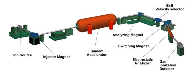
8 MV – primarily used for mass spectroscopy.
