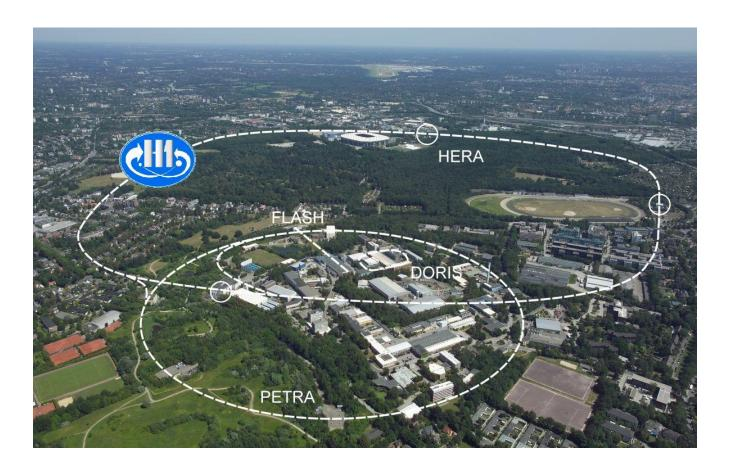
DORIS (1974-1993):  $e^+e^-$  collisions at  $E_{cm}=10~{\rm GeV}$ PETRA (1978-1990):  $e^+e^-$  collisions at  $E_{cm}=38~{\rm GeV}$ HERA (1990-2007): e-p collisions,  $E_{e^-}=27.5~{\rm GeV}$ ,  $E_p=920~{\rm GeV}$
