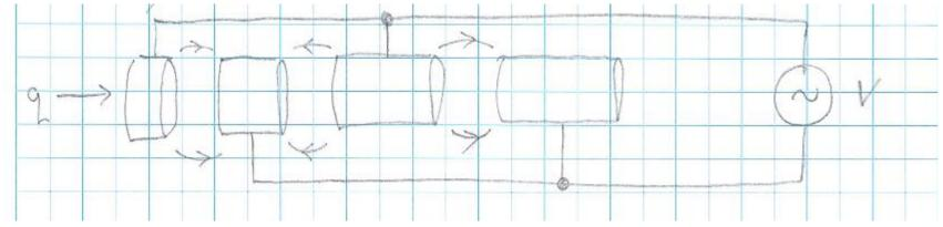
If the voltage source changes phase when particles are inside the cavities, then they will be accelerated in the gaps between the cavities.
