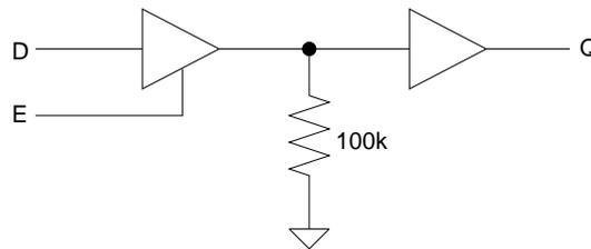
Write the truth table for  $Q$  as a function of  $D$  and  $E$ . What boolean algebraic operation does this implement?
