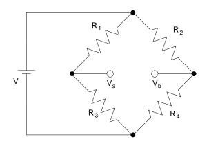
(a) Calculate the values of  $V_{\text{Th}}$  and  $R_{\text{Th}}$  needed for Thevenin's equivalent circuit for the voltage  $\Delta V = V_a - V_b$ .
