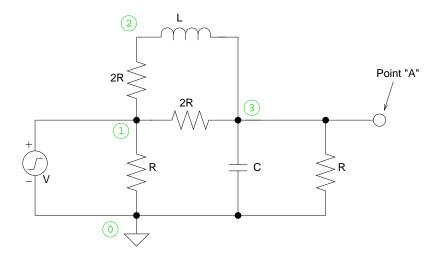
(a) If the voltage source makes a transition from 0 to V at t = 0, calculate the voltage at point "A" in the limit as  $t \to \infty$ .
