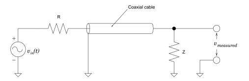
(a) With the input to the oscilloscope terminated with a Z = 50 Omega resistance to ground, calculate the measured voltage,  $v_{\text{measured}}$  in terms of  $v_{\text{in}}$ , R and Z, assuming  $v_{\text{in}}$  is a constant, ideal voltage source.
