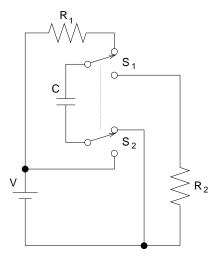
(a) Draw the equivalent circuit when the switches are in the position indicated in the diagram and calculate the potential difference that develops across the capacitor in the limit when  $t \gg 1/R_1C$ . (b) At some later time, the both  $S_1$  and  $S_2$  switched simultaneously. Draw the equivalent circuit and calculate the potential difference across  $R_2$  the instant after this event.
