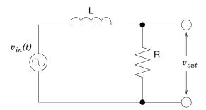
When  $v_{in}(t) = V_{in}e^{i\omega t}$ , the Thevenin equivalent circuit would consist of an ideal voltage source  $V_{\text{Th}}$  in series with an impedance  $Z_{\text{Th}}$ , both of which depend on the frequency,  $\omega$ .
