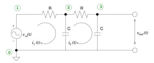
(a) Assuming  $v_{in}(t) = V_{in}e^{i\omega t}$ ,  $i_1(t) = I_1e^{i\omega t}$ ,  $i_2(t) = I_2e^{i\omega t}$  and  $v_{out}(t) = V_{out}e^{i\omega t}$ , solve the system of equations to determine  $I_2$  and show that
