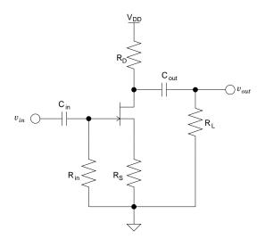
in which  $V_{DD}=15~\mathrm{V}$  and the parameters for the JFET are
