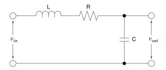
2. What inductance would be needed to make a second-order low-pass RLC filter with a cut-off frequency of  $f = 2\pi\omega_0 = 1$  MHz if a 10 nF capacitor was to be used? In principle, this filter could act as an RLC resonant circuit near this frequency. What value of R would ensure that the Q-factor for this oscillator is equal to 1?
