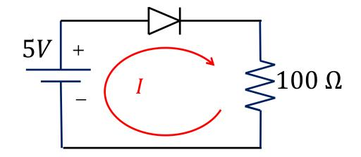
• The current in the circuit is  $I = \frac{5 \text{ V} - 0.727 \text{ V}}{100 \Omega} = 43 \text{ mA}$
