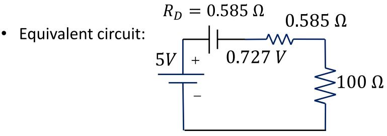
• Except for the change in potential across the junction, the diode has a very low resistance.
