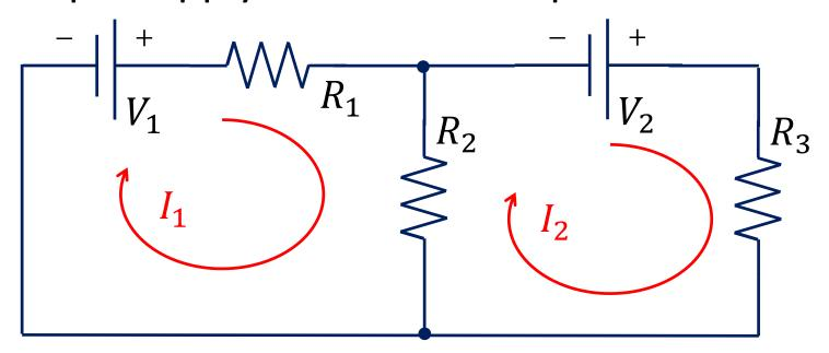
$$V_1 - I_1 R_1 - (I_1 - I_2) R_2 = 0$$
