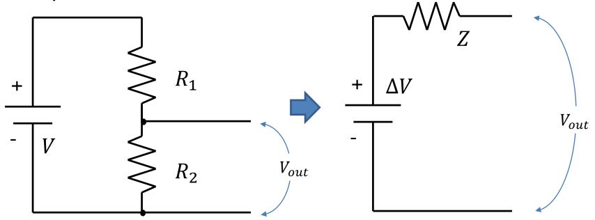
$$\Delta V = \frac{VR_2}{R_1 + R_2} \qquad Z = \frac{R_1R_2}{R_1 + R_2}$$
