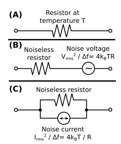
Example:  $R = 50 \Omega$ ,  $\Delta f = 1 \text{ Hz}$ ,  $T = 300 \text{ K} \Rightarrow v_{\text{rms}} = 1 \text{ nV}$
