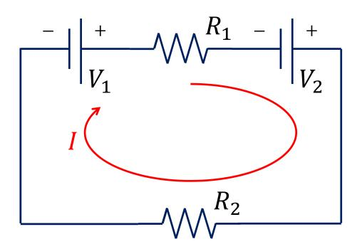
$$I = \frac{V_1 + V_2}{R_1 + R_2}$$
