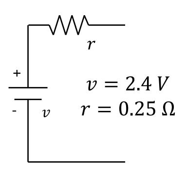
The model is only valid for a specific range of discharge currents, in this case maybe between 300 and 700 mA, and only when the temperature is 20 °C.
