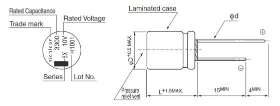
Short lead/black mark indicates the cathode (more negative terminal). But be careful: Sometimes the mark indicates the anode!
