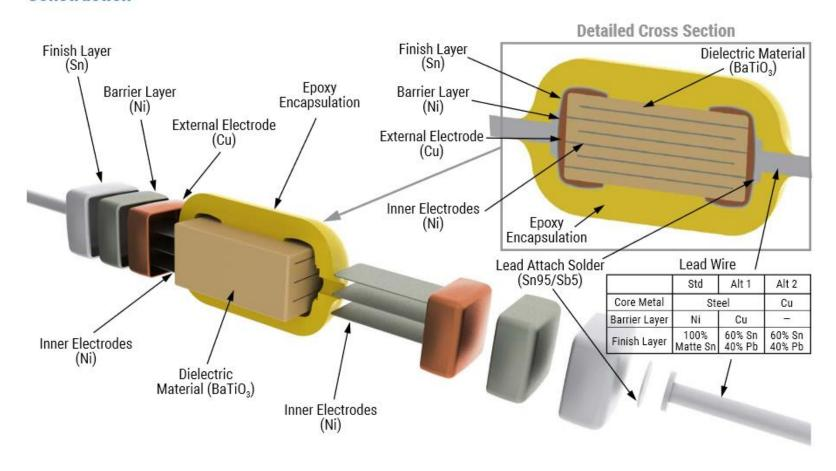
Ceramic capacitors are not polarized
