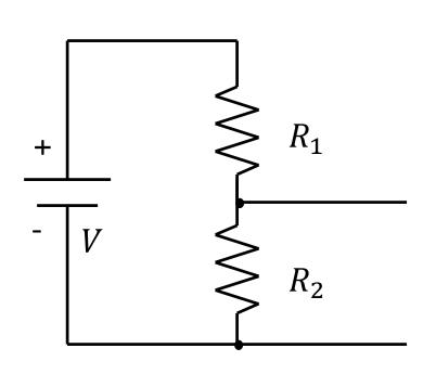
With no load applied, the current through  $R_1$  and  $R_2$  will be
