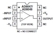
The AD8047 and AD8048's low distortion and cap load drive make the AD8047/AD8048 ideal for buffering high speed ADCs. They are suitable for 12-bit/10 MSPS or 8-bit/60 MSPS ADCs. Additionally, the balanced high impedance inputs of the voltage feedback architecture allow maximum flexibility when designing active filters.
