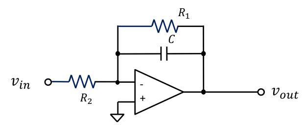
$$V_{out} = -V_{in} \frac{R_1}{R_2} \frac{1}{1 + i\omega R_1 C}$$
