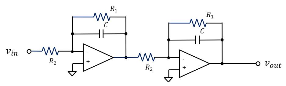
$$A = \left(\frac{R_1}{R_2}\right)^2 \frac{1}{1 + \omega^2 R_1^2 C^2}$$
