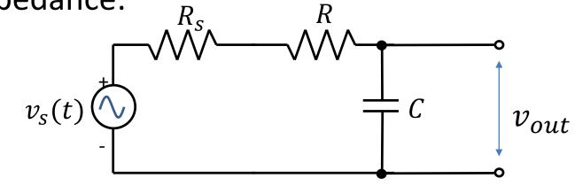
• As  $\omega \to 0$ , the output impedance of the filter circuit is  $R_s + Z$ . Increasing the number of filter stages also increases the output impedance.
