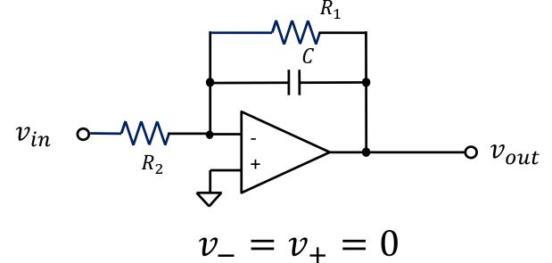
• Input impedance is  $R_2$ . This determines how much current will be drawn from the source.
