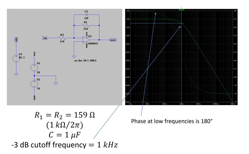
The property of having a low output impedance and an output that is isolated from the input makes it easy to analyze additional filter stages:
