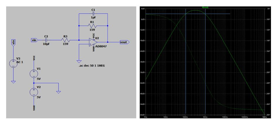
$$\omega_{-} = \frac{1}{R_{2}C_{2}} = 628.9 \ s^{-1} \rightarrow f_{-} = 100 \ Hz$$
