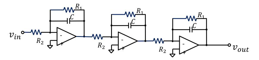
$$A = \left(\frac{R_1}{R_2} \frac{1}{\sqrt{1 + \omega^2 R_1^2 C^2}}\right)^3$$
