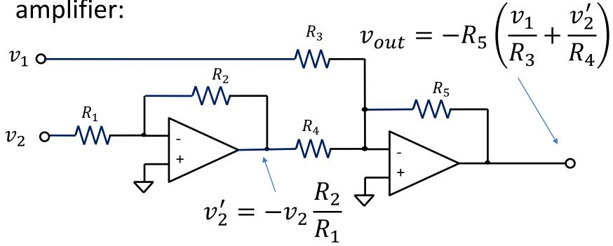
• If  $R_1 = R_2$  and  $R_3 = R_4$  then  $v_{out} = -\frac{R_5}{R_3}(v_1 - v_2)$
