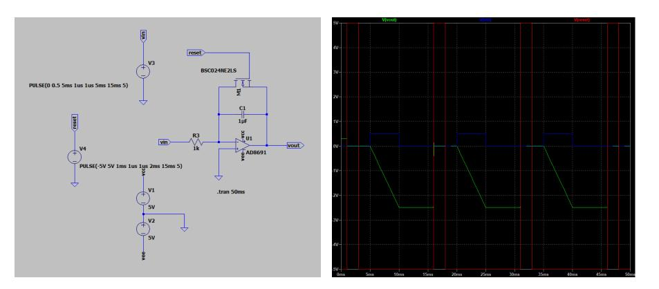
One annoying feature about MOSFET's is that the gate voltage is not compatible with most digital interfaces which range from 0 to 2.5, 3.3V or 5V.
