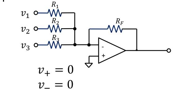
• No current flows into the inverting input.
