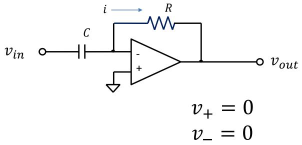
• But  $v_{out} = -iR$  where *i* is the current that flows through the capacitor.
