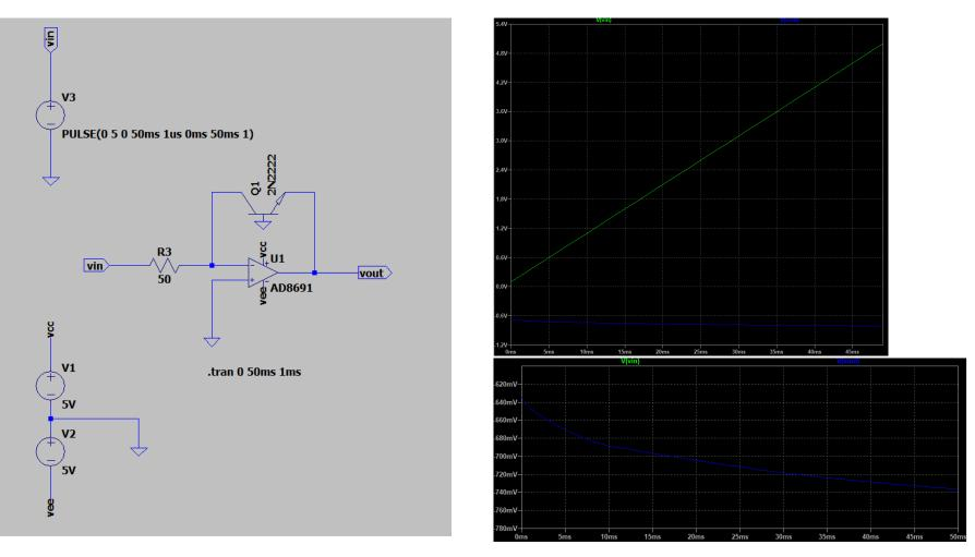
The dynamic range is somewhat limited and there is a significant voltage offset. These can be addressed by adding a summing amplifier as a second stage.
