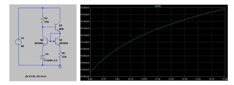
Now the output impedance is 35 k $\Omega$  but the collector of Q3 is at a higher potential with respect to ground.
