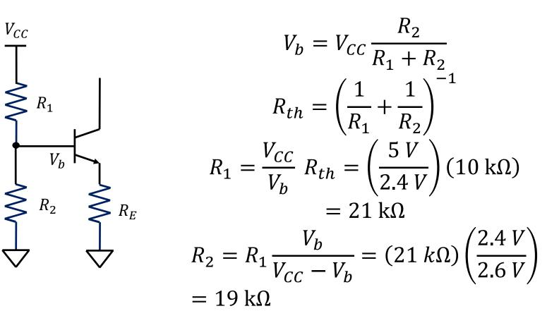
• These estimates provide a good starting point for simulating the circuit:
