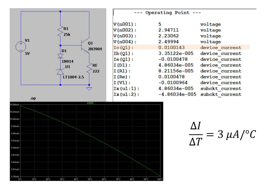
Better temperature compensation can be achieved by using exactly the same type of PN junction in the voltage reference circuit
