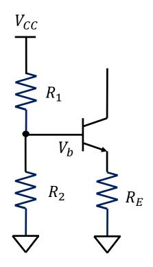
$$V_b = V_{CC} \frac{R_2}{R_1 + R_2}$$
