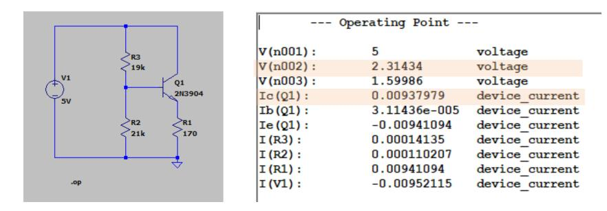
This is close... maybe raise the base voltage a little bit by increasing R2.  $R_2 = 24 \text{ k}\Omega \text{ gives } I_c = 10.075 \text{ mA.}$
