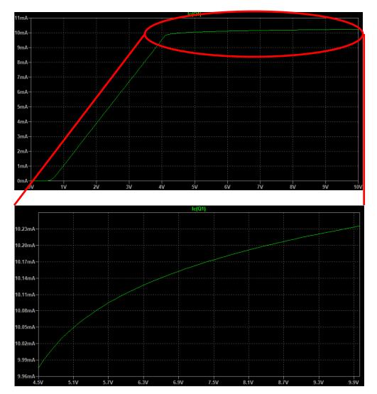
This is still not a perfect current source. The output impedance is about  $20 \text{ k}\Omega$ .
