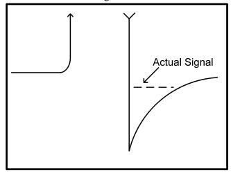
When it is necessary to observe small voltages shortly after a large voltage, a limiter must be used to prevent the large voltage from overloading the scope.
