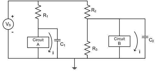
The capacitor provides the low impedance path and the resistor inhibits the current from going onto the voltage line where it could interfere with the other circuits.  $R_1$  and  $C_1$  also act as an AC voltage divider to prevent noise on the voltage line from affecting circuit-A.  $R_1$  can be replaced by an inductor if low DC resistance is needed between circuit A and
