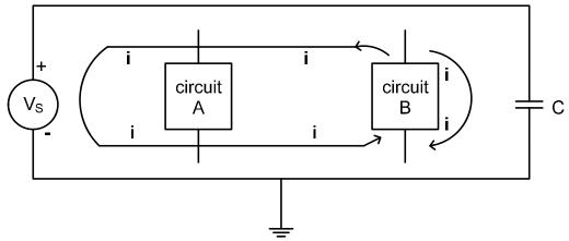
At high frequency, however, the inductance of the long wires creates impedance, and the long path serves as an antenna to send and receive high-frequency noise. A by-pass capacitor from the voltage line to common solves the problem by providing a short, local path for the high-frequency current, it also should have a by-pass which provides the shortest practical closed loop. The capacitor should be large enough that it presents negligible impedance for the frequency range it must handle.
