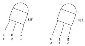
The numbers indicate correspondence between parts. For example, the emitter (1) of the BJT has the same function as the source (1) of the FET. Notice that the pin order is quite difference for the BJT and FET, hence you must rearrange a circuit when these transistors are interchanged.
