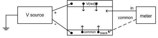
circuit through the red terminals. The negative terminal of the source must be connected to the circuit common, which is the black terminals and the metal box (see GI-1.2). A voltage in the circuit can not be measured by connecting the input lead of the meter to a point in the circuit. The meter-common and circuit-common also must be connected as shown by the dotted line.
