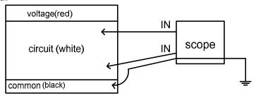
(Although this is satisfactory for our lab, a connection to common should be used for each probe when high-frequency signals are observed). The scope is grounded through the third wire of the AC plug to protect against leakage in its power supply. The scope common is grounded through the scope, hence the circuit common also is grounded through the scope.
