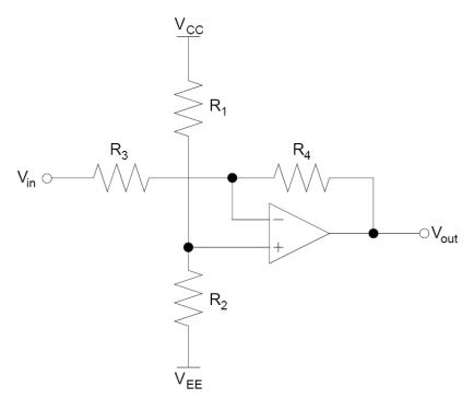
(a) Derive constraints that  $R_1$ ,  $R_2$  and  $R_3$ ,  $R_4$  must satisfy in order to implement the following linear transformation of the input voltage:
