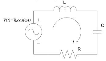
(a) Calculate the frequency,  $\omega$ , of the voltage source that will maximize the power drawn by the circuit.
