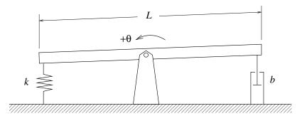
(a) When in equilibrium, the beam is horizontal. Write the differential equation that describes the small angle  $\theta$  measured with respect to the equilibrium position with  $+\theta$  in the direction shown on the figure. The moment of inertia of the beam about the fixed axis is  $I = \frac{1}{12}ML^2$ .
