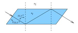
Light initially polarized at 45° has equal components of its electric field parallel and perpendicular to the plane of incidence. Show that these two polarization components will emerge from the Fresnel rhomb with a phase difference of  $3\pi/2$ .
