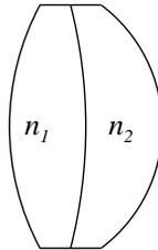
If the front surface has radius of curvature  $R_1$ , the interface between the two lenses has radius of curvature  $R_2$  and the back surface has radius of curvature  $R_3$ , calculate the focal length of the assembly using the thin lens approximation.
