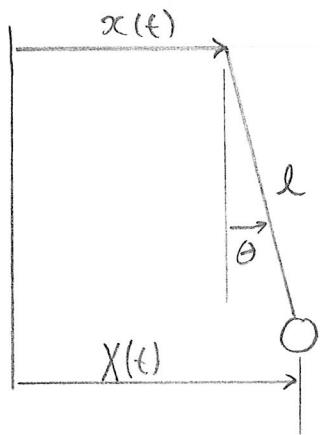
In this diagram,  $X(t)$  is the position of the mass in an inertial reference frame. It is related to  $x(t)$  and  $\theta(t)$  by
