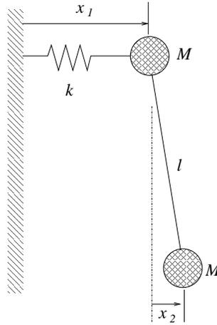
The top mass has displacement  $x_1$ , measured with respect to its equilibrium position, and the bottom mass has displacement  $x_2$ , measured with respect to the top mass.
