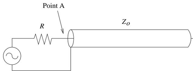
The far end of the cable is an open circuit and the source and cable impedances are matched so that  $R = Z_0$ . If signals propagate in the cable with a speed  $v$ , what is the lowest frequency that will result in a maximum voltage, measured at point A?
