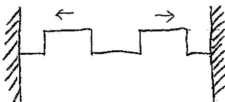
At time  $t = 3\text{s}$  the pulses have reflected from the ends, and are now inverted:
