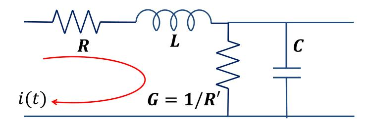
• It is convenient to describe the resistor that is in parallel with the capacitor in terms of its conductance, G = 1/R'.
