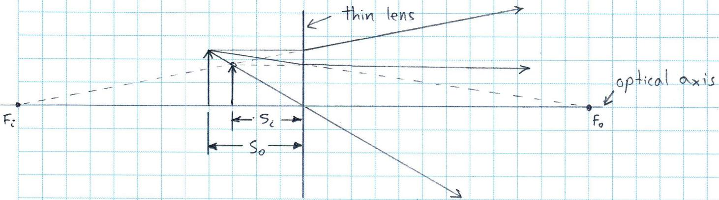
$$\frac{1}{s_o} + \frac{1}{s_i} = \frac{1}{f} \Rightarrow s_i = \left( \frac{1}{f} - \frac{1}{s_o} \right)^{-1} = \left( \frac{1}{-30 \text{ cm}} - \frac{1}{10 \text{ cm}} \right)^{-1} = -7.5 \text{ cm}$$
