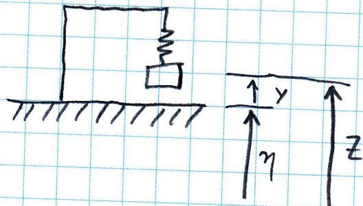
where  $z$  is in an inertial reference frame
