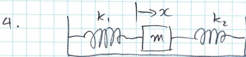
When the mass is displaced from its equilibrium position by a distance  $x$ , the force acting on it will be
