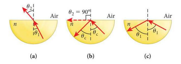
Critical angle  $\theta_C$  defined by  $n \sin \theta_C = 1$ . At angles greater than  $\theta_C$ , all light is reflected from the surface.
