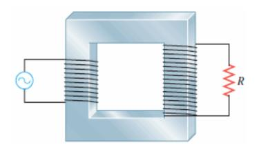
Equal flux  $\Phi$  through both windings.
