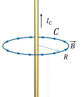
• The path length element is also azimuthal:  $d\vec{\ell} = d\ell\hat{\varphi}$
