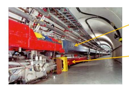
Normal dipole magnets  $B \sim 1 T$
