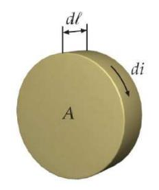
Magnetic dipole for a current loop:  $\vec{\mu} = A \; I \; \hat{n}$
