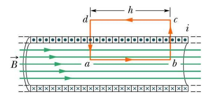
$$\oint_C \vec{B} \cdot d\vec{\ell} = \int_a^b \vec{B} \cdot d\vec{\ell} + \int_b^c \vec{B} \cdot d\vec{\ell} + \int_c^d \vec{B} \cdot d\vec{\ell} + \int_d^d \vec{B} \cdot d\vec{\ell} = \mu_0 I_C$$
