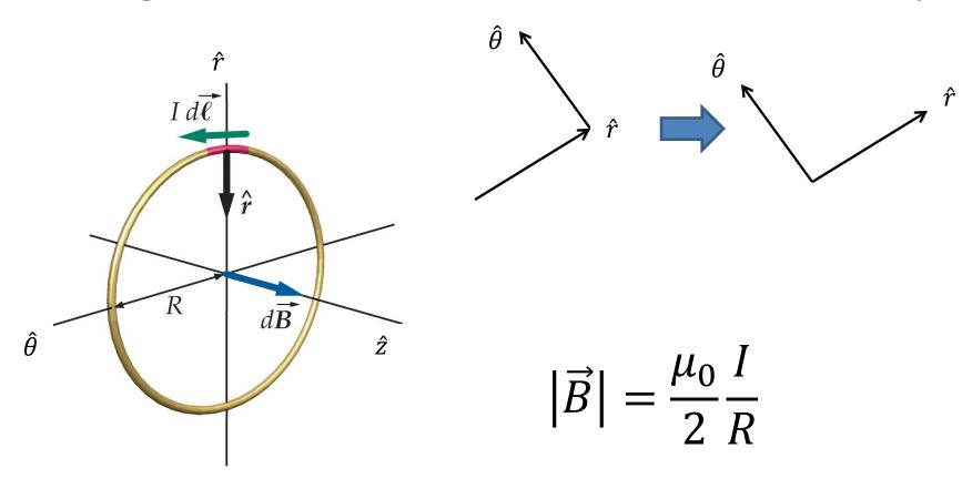
Magnetic field on the axis of a current loop
