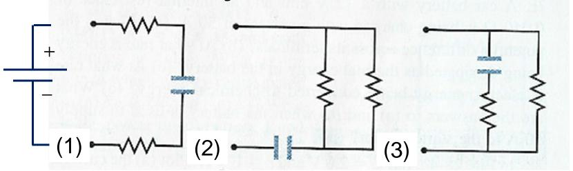
As  $t \to \infty$ , the capacitor acts like an open circuit: no current will flow through it.
