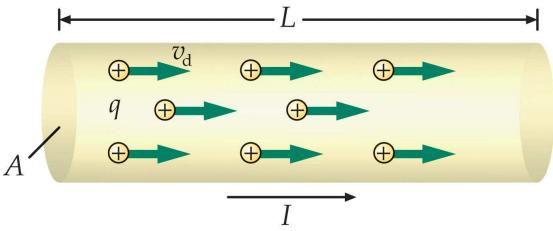
Force on one charge:  $\vec{F} = e \ \vec{v}_d \times \vec{B}$
