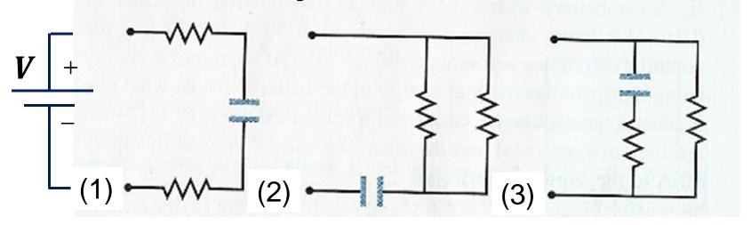
The figure shows three section of circuit that are to be connected in turn to the same battery via a switch. The resistors are identical, as are the capacitors. Rank the sections according to the final charge  $(t \to \infty)$  on the capacitor.
