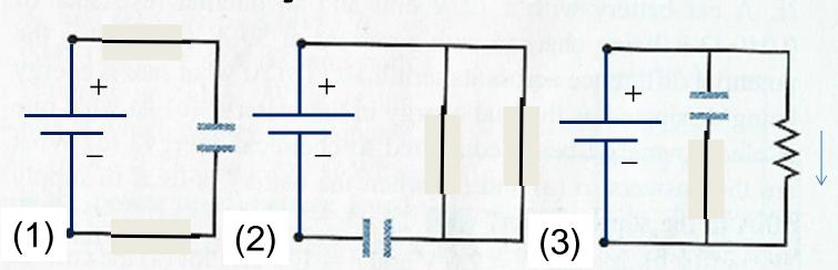
In circuit (3), current still flows through the resistor, but this doesn't change the potential across the capacitor.
