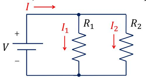
The voltage across each resistor is equal.
