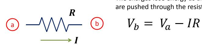
The charges lose energy as they are pushed through the resistor.
