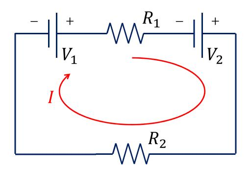
$$I = \frac{V_1 + V_2}{R_1 + R_2}$$
