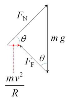
•  $F_F$  is zero when the curve is banked correctly.
