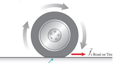
If the tire turns faster, it pushes back harder on the road. The road in turn pushes forward on the tire, causing the car to accelerate to the right. (c) The tire is moving to the right and turning slower.
