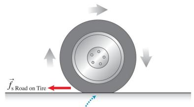
If the tire turns slower, it pulls forward on the road and the road pushes back on the tire, exerting a force that slows the car, causing it to accelerate backward.
