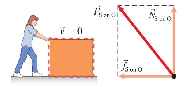
The force of the surface on the block is considered as two forces: the normal force  $\vec{N}$  and the friction force  $\vec{f}$ .
