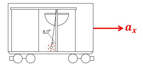
• A train car moves with constant acceleration  $a_x$  causing a pendulum inside it to swing to an angle  $\theta=8^\circ$  with respect to the vertical. What is the acceleration,  $a_x$ ?
