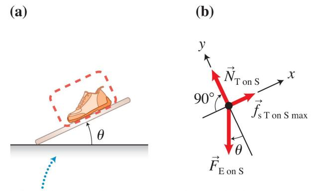
There is a maximum tilt angle at which the static friction has its maximum value just before the shoe slides.
