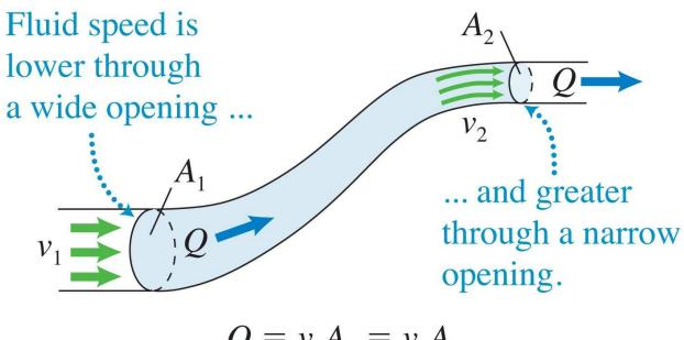
$$Q = v_1 A_1 = v_2 A_2$$
