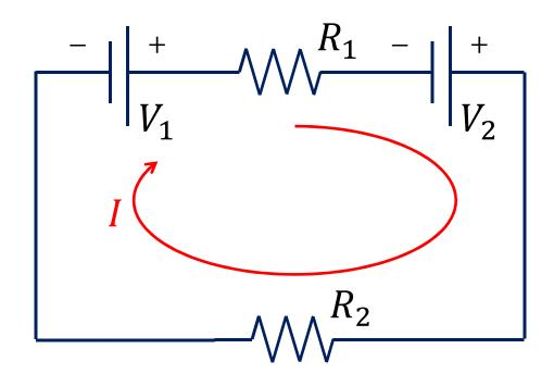
$$I = \frac{V_1 + V_2}{R_1 + R_2}$$
