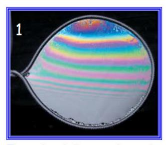
The color indicates where the wavelength and <u>local</u> film thickness satisfy constructive interference criteria.
