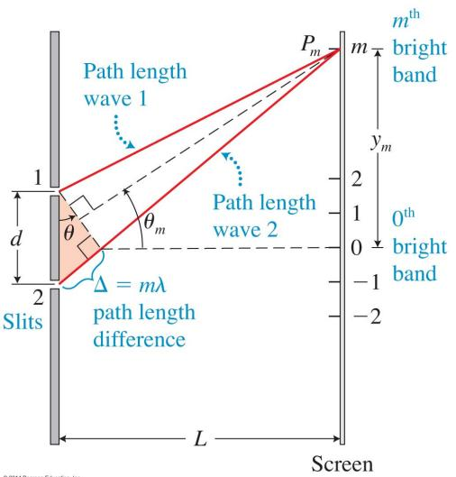
When the initial phase is the same, the path length difference is:
