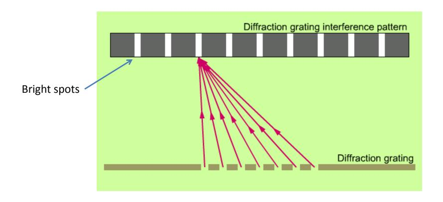
Bright spots on a viewing screen are produced by the constructive interference of light from many, many slits.
