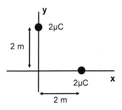
5. Two point charges are located as shown in the figure to the right. What is the electrostatic potential at the coordinate origin?
