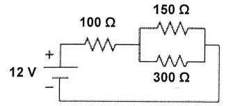
15. In the circuit above, what is the power dissipated in the 100  $\Omega$  resistor?
