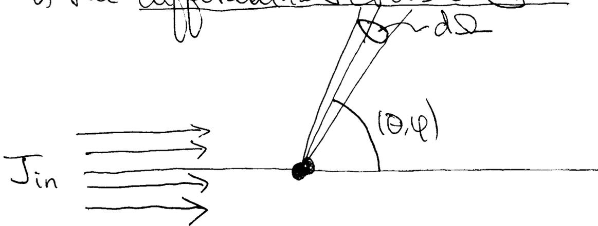
Suppose the particle detector is located in the direction  $(\theta, \varphi)$  at a distance  $r$  from the target and well outside the incident beam of particles. If the detector subtends solid angle  $d\Omega$  it will receive  $dn = J_{in} \sigma d\Omega$  scattered particles per unit time. The area of the detector is  $(r^2 d\Omega)$  then we have a flux of outgoing scattered particles at the detector of
