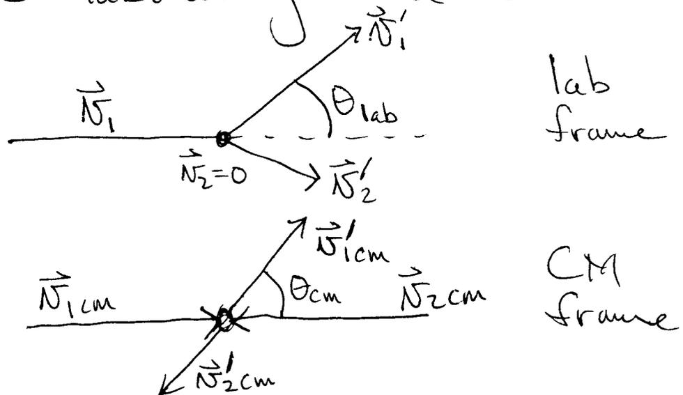
In the lab frame the incoming particle has mass  $m_1$ , velocity  $\vec{v}_1$ , while the target particle of mass  $m_2$  is at rest. The velocity of the center of mass is then
