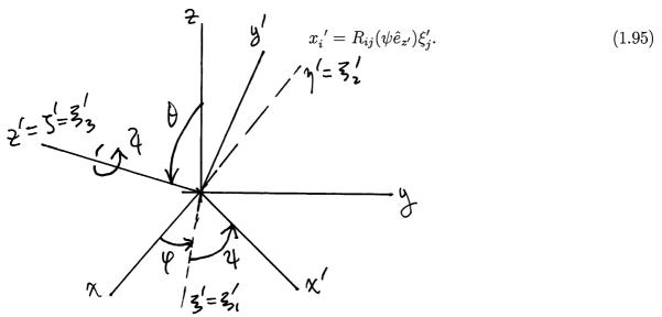
The Euler angles  $(\theta, \varphi, \psi)$  completely specify the rotation. Thus we can label R by  $R_{ij}(\theta, \varphi, \psi)$ . So we have
