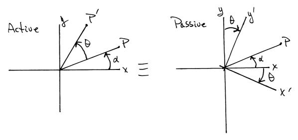
(Active View)Rotate P CCW( $\theta$ ) to P' axes fixed.
