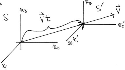
So  $x_i' = x_i - V_i t$  where  $\vec{V} = \text{const.}$  Here we have assumed that time is absolute
