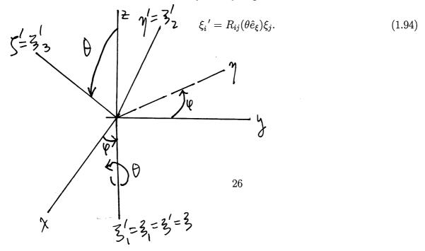
Finally rotate about the  $\zeta'$ -axis by angle  $\psi$
