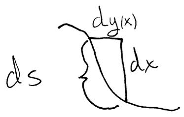
$ds = \text{distance along curve travelled in time } dt$
