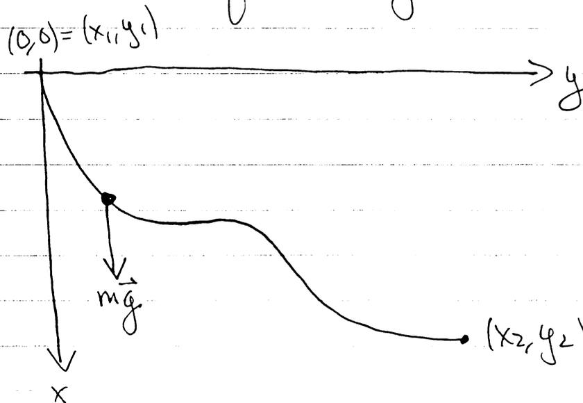
Suppose we ask the question: What shape should the curved wire be so that the particle initially at rest at the origin arrives at  $(x_2, y_2)$  in
